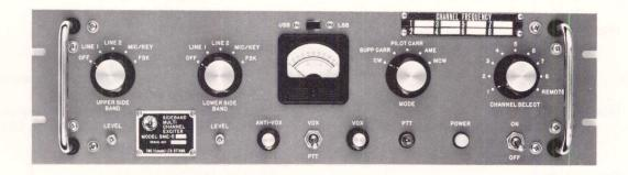
The SME-5 is a fully transistorized, eight channel ISB exciter with a frequency range of 2 to 30 MHz. It provides up to 100 milliwatts PEP output as drive power for an associated linear amplifier. Capable of operating in all modes normally encountered in this range, it is particularly useful as a single sideband device for voice, teletype, facsimilie or other type of communication.
