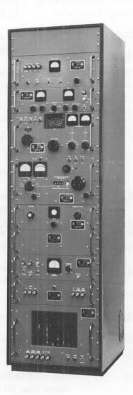
TMC Model SBG-1L (AN/URA-41) and Model SBG-1M are synthesized oscillator/exciter units that provide highly stable 100 cycle incremental tuning in the VLF/LF/HF portions of the frequency spectrum. Both units feature frequency stability and resettable accuracy of 1 part in 10<sup>8</sup> for 24 hours.
