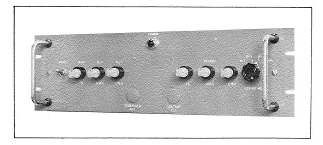
The TMC Model ISK, Isolation Keyer, is a transmitting type keying device designed to provide isolation between the keying line and its associated transmitter. It will accept inputs of 50v, 100v, 20ma, and 60ma.
