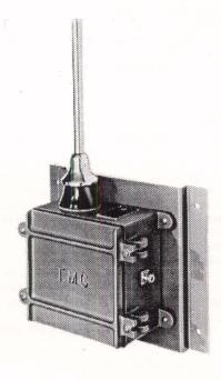
All AVA antenna components are enclosed in a rugged, weatherproof case constructed of cast aluminum alloy and available in standard or EMI/RFI shielded versions. Except for the tongue and groove gasket channel, the external surfaces of the enclosure are painted and internal surfaces are coated with a clear iridite for maximum conductivity and protection.
