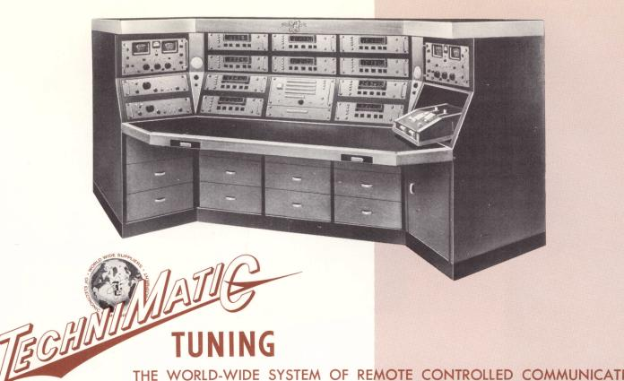
This console permits an operator to tune both transmitters and receivers remotely to frequencies and various modes of operation on an automatic and pre-programmed basis by means of pre-cut tapes, cards, memory systems or manual selection and provides a readback of information to the operator showing him that the selected tuning functions have, in fact, been performed.
