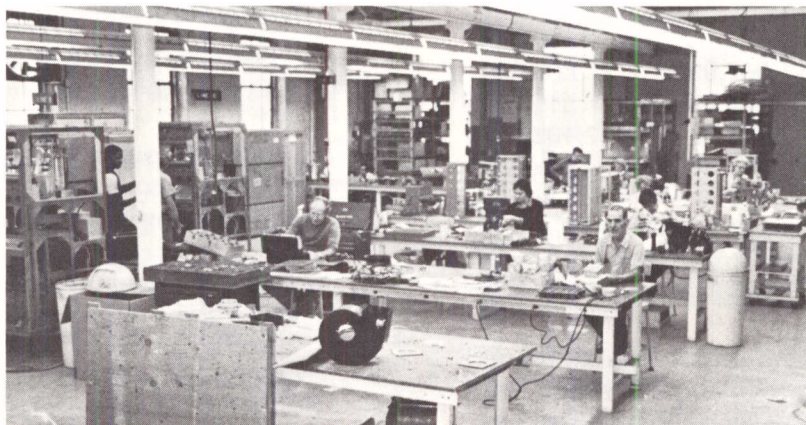
Production area where transmitters are completely disassembled and rebuilt.
