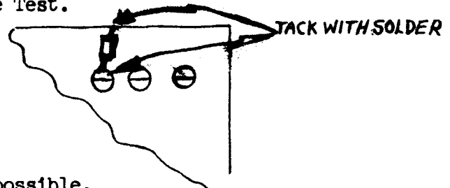
Suggested mounting of resistors for Frequency Response Test.
