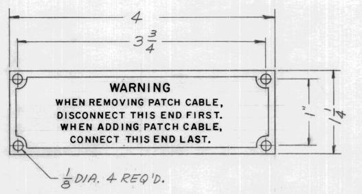
NAMEPLATE TO BE MANUFACTURED IN ACCORDANCE WITH MIL-P-15024B, TYPE, A 17 JAN. 1957.
