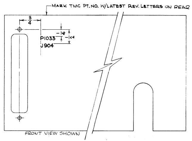
MARKING PROCESS: AS PER TMC SPECIFICATION S-727.
