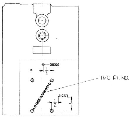
MARKING PROCESS: AS PER TMC SPECIFICATION S-727.
