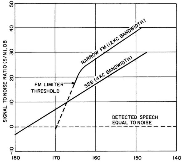
ATTENUATION BETWEEN TRANSMITTER AND RECEIVER, DB
