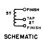
**REVISIONS**  $\triangleleft$ SYM DESCRIPTION DATE E.M.N. NO. B/M: IT. (6) SYM. WAS GREEN; SCHEM; ST WAS 8T; ZT WAS 3T; WINDING PROCEDURE; #1, 5 TURNS WAS 8 TURNS; TAP AT 2 WASTAP 2-12-65 13300 AT 3; ELEC. SPECS: START-FINCH, .27 WAS .34; START-TAP, 10 WAS.11 A-3157
